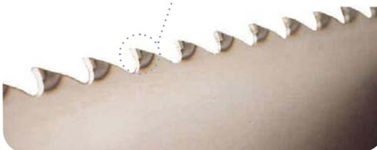
*EPS use high quality Bohler Uddeholm steel to manufacture wide band saws in a range from 60mm to 360mm wide with the blades tensioned to your specifications. Your band saws can be supplied ready to run or just toothed and joined. The teeth can be produced in a constant or in a vari-pitch format. The cutting teeth can be Swaged and Shaped, or Stellite Tipped for a more durable and longer lasting cutting edge.*
